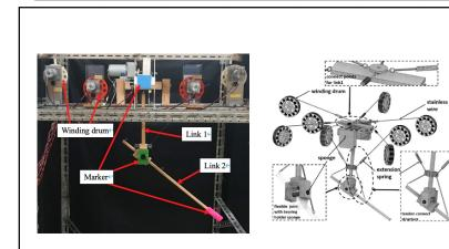
A soft robot joint was made using a rubber bearing holder. Elastic tendon drive method enables simple joint mechanism without motors, reductions, and encoders.
