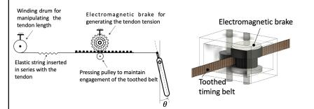
Kinematics without using joint angles is useful when controlling this type of soft robot, because the joint angles are not strictly determined due to the swing motion of the joint axis. Content:
